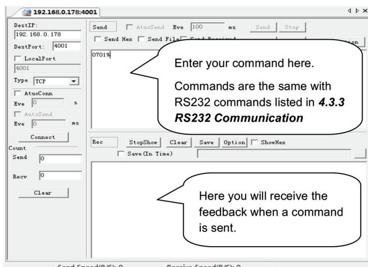
FIGURE 7-4. CONTROL INTERFACE OF TCPUDP
