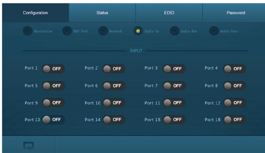
FIGURE 7-12. CONFIGURE AUDIO INPUT
