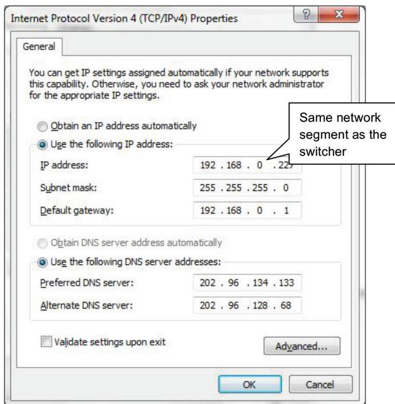
FIGURE 7-1. MATRIX SWITCHER CONTROLLED BY A PC WITHOUT ETHERNET ACCESS
