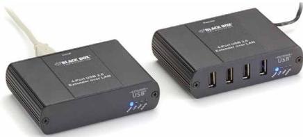
Switchable High-Speed USB Extenders (EMD100USB)
